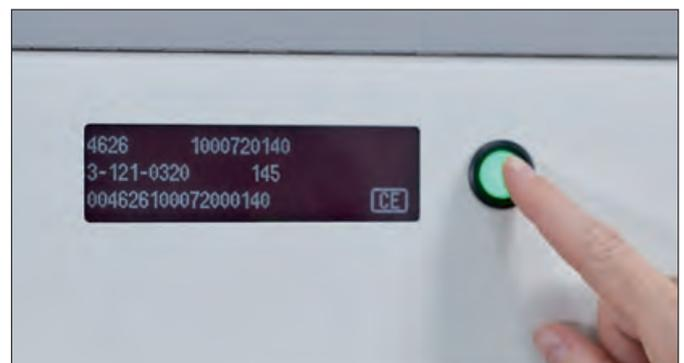
The Hänel digital picking display indicates where the requested item is located in the system and also provides additional information about the item and its storage position
