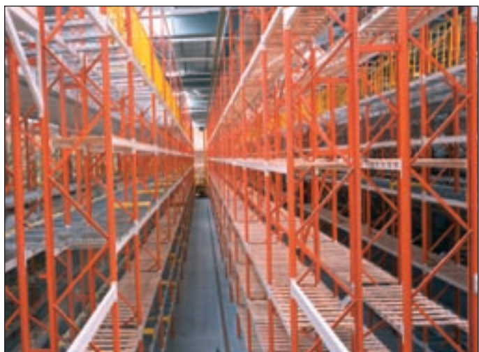
Special design: levels with decking and integrated roller tracks
