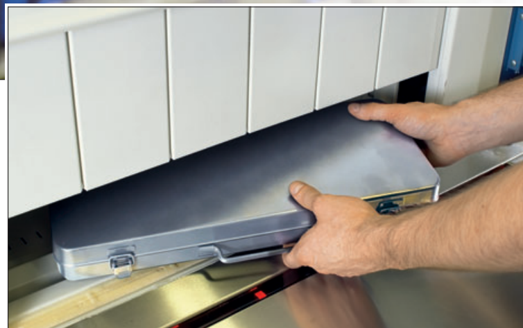
Fully automatic compartment doors for the retrieval of different-sized parts
