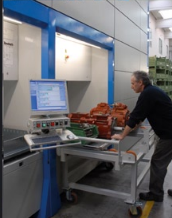
RETRIEVAL retrieval operation and goods positioning on trolley
